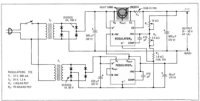
**Variable supply.** This power supply, which employs two IC voltage regulators, produces a regulated output voltage of between 0 and 30 V. REGULATOR<sub>1</sub> provides the bias voltage for REGULATOR<sub>2</sub> so that the latter device can operate with respect to a common ground. The lowest regulated output voltage, then, is approximately zero, rather than the reference voltage of REGULATOR<sub>2</sub>.
